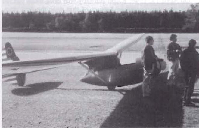
Baby Bowlus with its usual rudder markings. Hawley Bowlus designed it using the wing of the Grunau Baby on a plywood pod and a steel tube boom bought from a hardware store.
