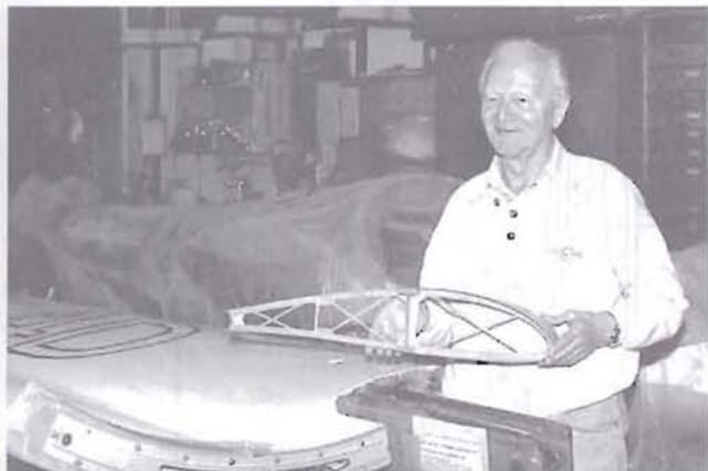
Figure 8 : Heinz Hinz with a section of the D 28 wing structure. In the foreground the wing root and flap track of the D 40, a more recent design of the Akaflieg Darmstadt.
