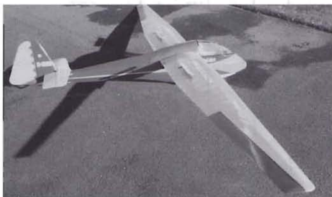
Peter Saunders' model Scheibe L. Spatz of 1/3.83 scale giving a span of 12ft 10ins and weighing 8lb 12 oz. Compare it with the original on page 35. Photo Peter Saunders.
