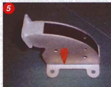
Check the Beak and Operating Lever bushes for excessive wear by Rocking the Beak and Lever laterally.
