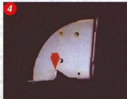
and carefully inspect the Casing Mounting Lugs for cracks and distortion. This may require the removal of protective treatment that must be replaced:
