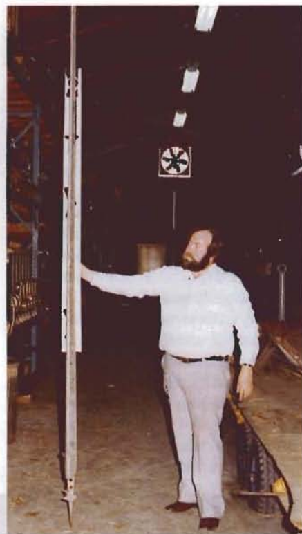
Bob Storck, former archivist for the Vintage Soaring Assn. (USA) shows the wing tip drag rudders of the Horten IV.
