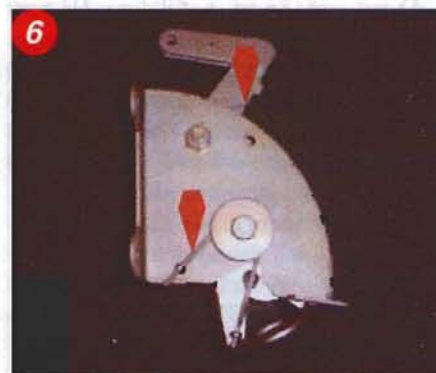
Visually inspect the springs for distortion and signs of impending failure.
