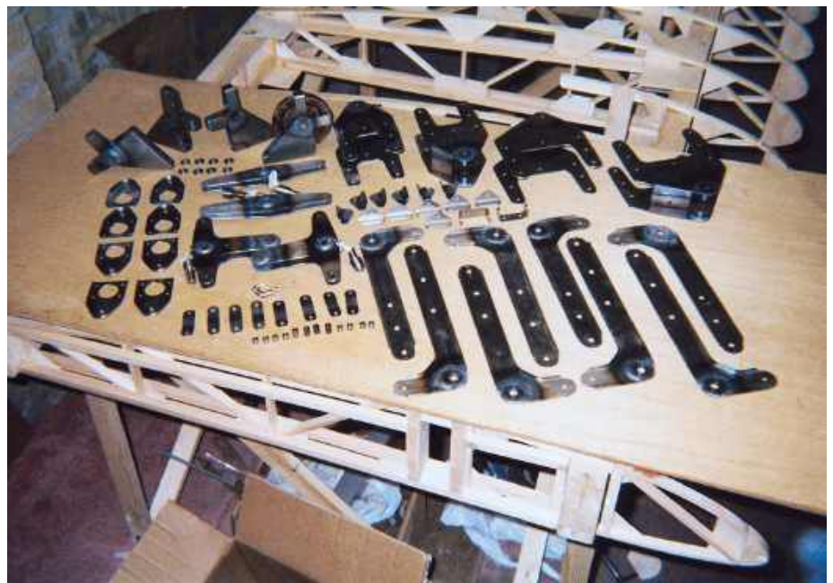
Above: steel fittings, prior to painting
