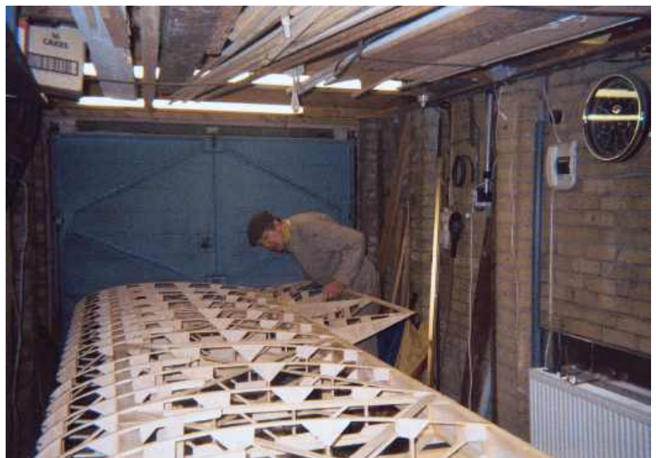
Below: aileron being offered up to starboard wing panel. Photos: Martin Francis
