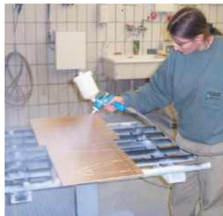
Top: rib template, with battens and fillets installed, ready for glueing. Above: impregnating the templates. Below: rib after glueing.
