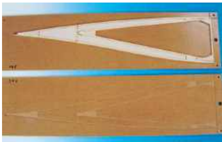
Above: template with finished rib. Below: final grinding of rib.
