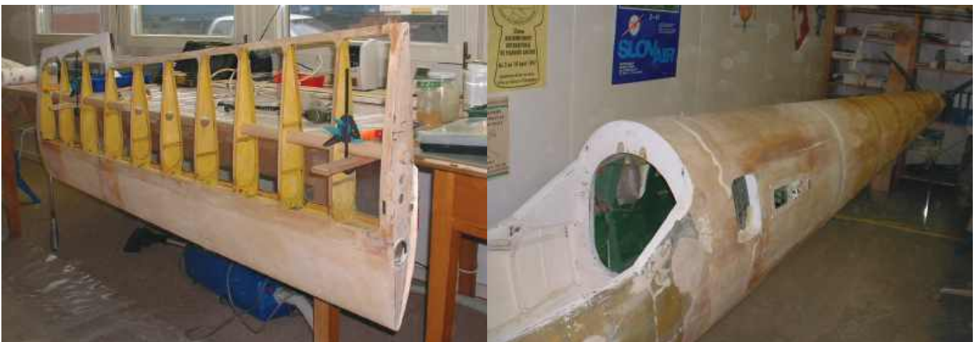
Below: the very precisely constructed V-tail of the Standard Austria S, HB-1299. The wooden fuselage of the HB-1299 after the remove of four (!) different coats of paint.
