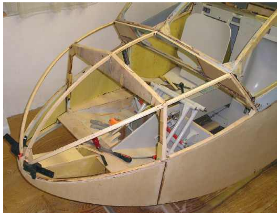
Below: Repairs to the nose Top right: 'Hangar flying' in the
