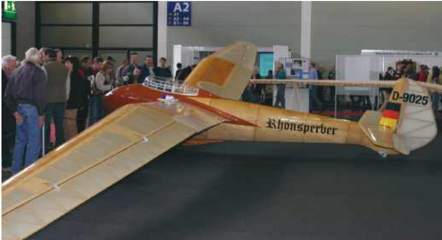
Left: RHOENSPERBER D-9025. This type was designed by Hans Jacobs and first flew with great success in 1935 breaking many National and International records. It was designed with a shoulder wing to give pilots more visibility as there had been some collisions during the 1934 Rheon Contest. This one was recently built by Otto Grau. 100 were originally built by the Flugzeugbau Schweizer. Now, only two remain airworthy in the world.
