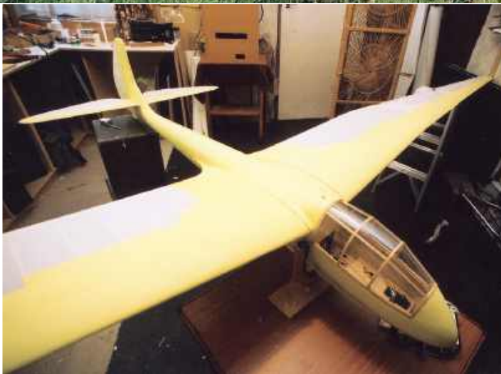
Right: Almost complete. Above: Ready to Go! Span: 5m; Scale: 1:3.5; AUW: 19lbs; Function: rudder, elevator, ailerons, brakes Profile: Quabeck 3.5/12 15%-12% Washout 2deg. Photos: Paul Broome
