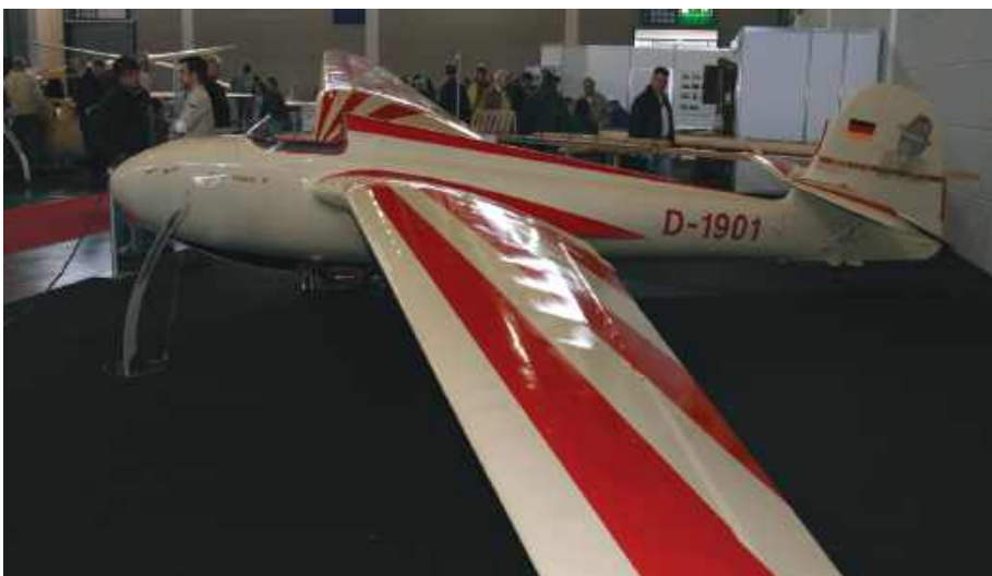
Above: HABICHT D-1901. The prototype flew in 1936 as a possible contender for Olympic aerobatic contest. This one was recently built by the Zahn family, Clemens, Walter and Christoph. Christoph flies it doing fine aerobatics. He says that it climbs like a Ka-8 at 70 kph and yet is cleared for a VNE of 250 kph. Designer was Hans Jacobs.
