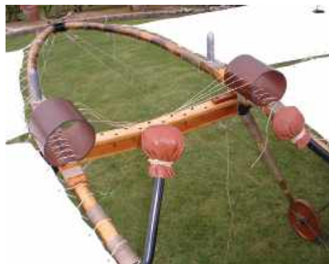
Top left: burning the midnight oil fitting the fabric Above: leather arm & shoulder supports, Above right: there are 140 separate wires to support the glider
