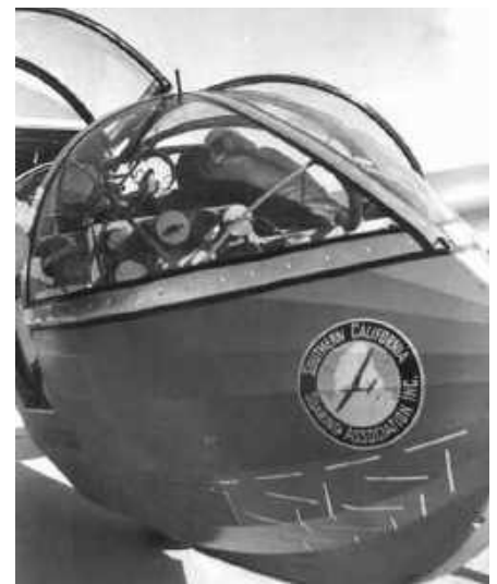
Close up of aluminium strips glued onto fuselage to give a better radar signature. Photo: Larry Edgar via Simine Short
