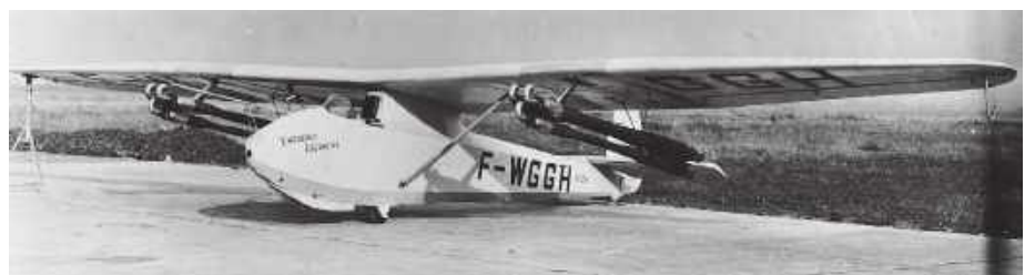
Left: Emouchet SA 604 'Escopette' with four pulse jets modified in during 1950 to see what minimum power could get it airborne.
