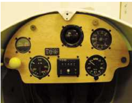
Top: fuselage of the Olympia Meise HB 384 in the workshop of Thomas Fessler Above: the tail of the Meise did not fit into the small workshop of Thomas Fessler Below: the new instrument panel of Meise HB 384. Take note of the FLARM (collision warning equipment). Photos: Thomas Fessler
