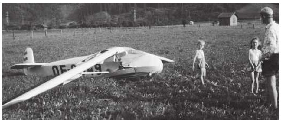
Below: the H.17B's wing trailing edge drag flaps could cause the H.17b to stall and crash if lowered with insufficient air speed, as appears to have happened to this H17B in Austria
