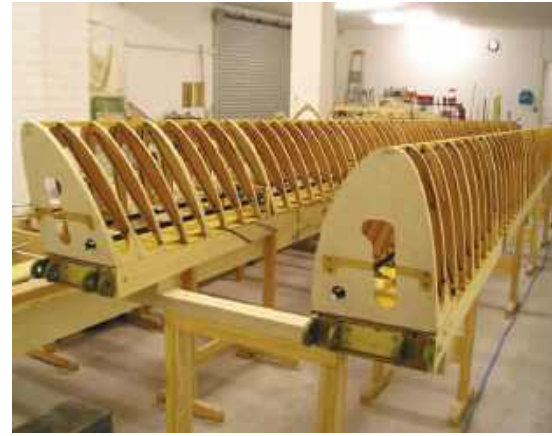
Photos show the assembly of the Horten IVA's wings making good progress at Sascha Heusers
