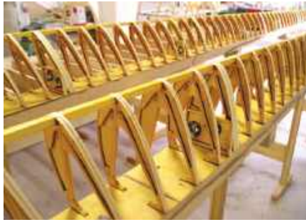
Photos show the assembly of the Horten IVA's wings making good progress at Sascha Heusers
