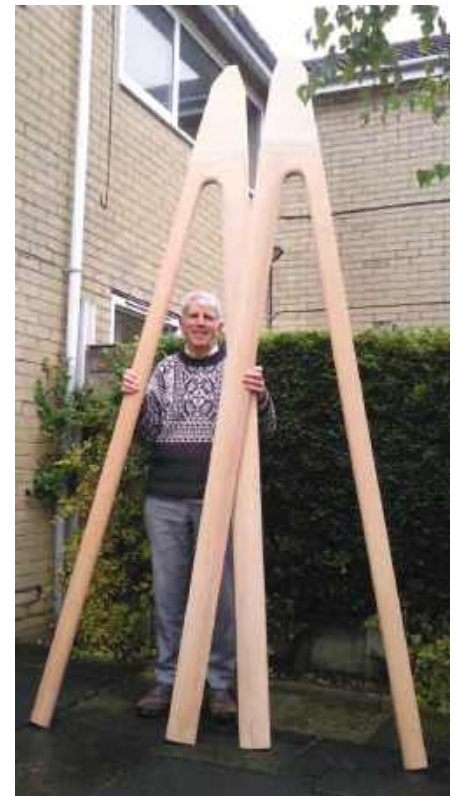
Right: Martin Francis with the Struts proper, a laminated structure, using Douglas Fir
