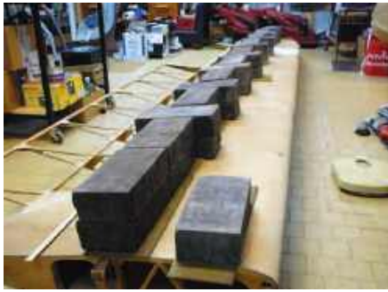
Top: Hütter 17 rigged hanging upside down ready for wing-loading test. The wooden struts, showing woodworm-holes will be replaced later by perfectly fitting metallic Slingsby-struts.
