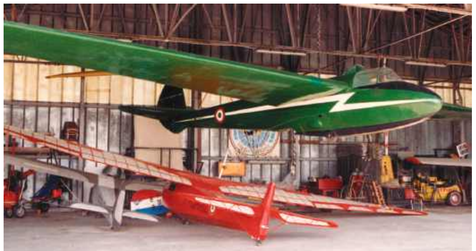
Top: Cattaneo RR Right: Canguro Palas in Pavullo (Note the aircscoop over the canopy in open position) Above: classic configuration of Mantelli's design: central egg-shaped body, two tail booms carrying the empennages with a single central fin and rudder.
