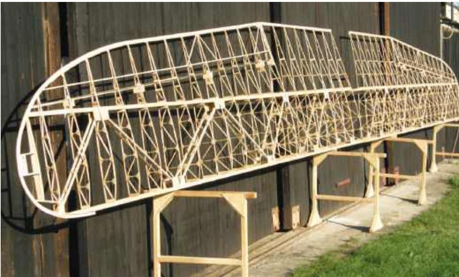
*Above: the "Sedy vlk" (Grey Wolf), whole structure of wings, tail units and fuselage sections are finished in the present.*
