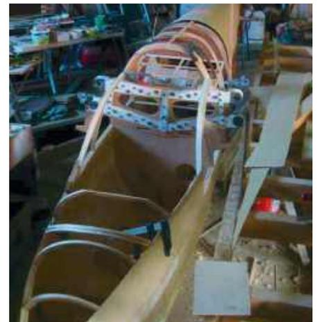
**Above: Minimoa front cockpit activity – the canopy frame is in place and will be ply covered when the nose is covered.**
