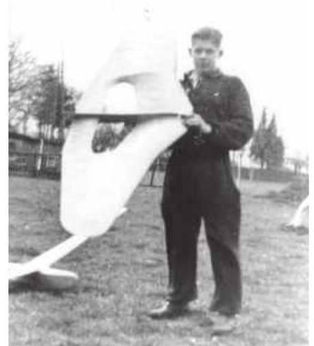
Herbert Guckel in the mid 1930's in Grunau with his first "Flying Wing". The centre keel worked as a stabilisor. The model's flight characteristics were described as excellent.
