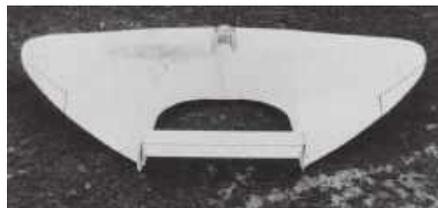
Herbert Guckel constructed the G-1 between 1943 and 1944 on the basis of his experimental experiences as he never had an Engineering education. The glider was equipped with split flaps on the wings' upper surface, with a wheel and two skids.
