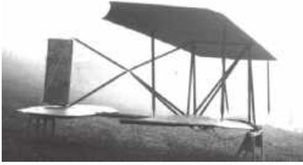
have a fabric cover intrados. According to the instructions, the fabric could be obtained from any cloth shop. Eugen also recalled that a moving vertical fin was added to the glider but that it did not perform as expected.
