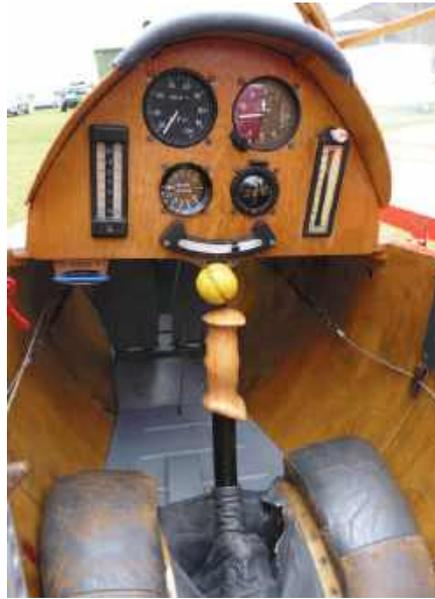
***Space in most old gliders is far more restricted than in modern gliders, so to find strong attachment points to fit a battery and transponder that does not restrict the pilot would be very difficult.***
