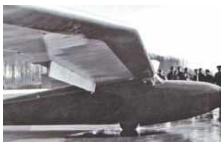
Above: prototype with high mounted wing and under-wing brake flaps. Below: later rudders were enlarged like the one on the left.
