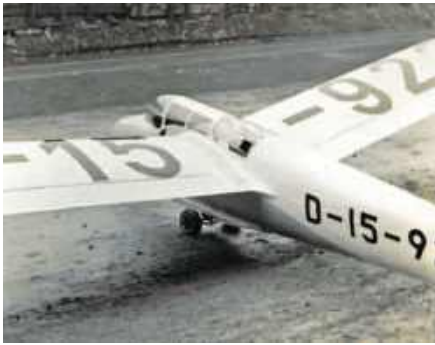
Top right: an early Minimoa for export, with the high mounted wing and all flying tailplane. Above: the two seater, the view from the rear cockpit was seriously restricted.
