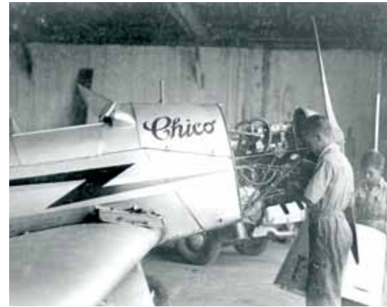
Bücker Student Chico receives attention. The engine is completely exposed once the panels are removed. Author's collection.
