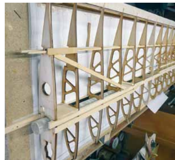
The Grunau baby's wings: laser cutting of parts much in evidence
