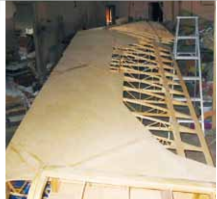
Spar ready for last ply webb. Spar constructed on bent table ready to close.
