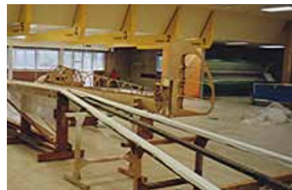
Main spar jigs at Soesterberg
