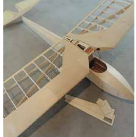
The wing skins have been added and some internal wiring done for the aileron servos, one in each wing. The elevators are skinned and covered with heat. Photo: Martin Simons
