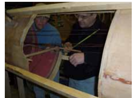
IOC Olympia 2b fuselage is jiggged up ready for new wood to be spliced in.
