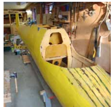
The fuselage now fully repaired, awaits controls and fabric. Photo: Ove B. Hillersborg
