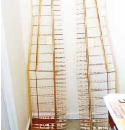
The wings also went together easily. The modified ailerons, not yet skinned, are evident here. Photo:: Martin Simons
