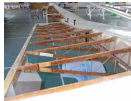
Fabric of MG-19 removed, ready for recovering.
