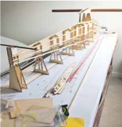
The simple jigging system and the pre cut formers fitting the longerons exactly, made the assembly of the fuselage very simple Photo:: Martin Simons
