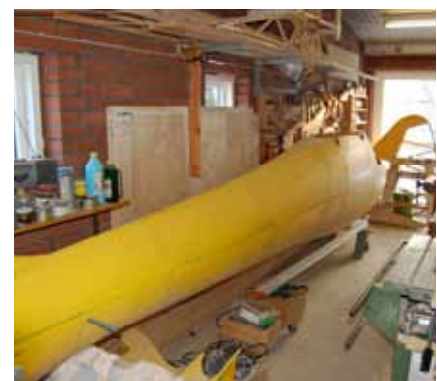
Rear view of the completed fuselage. Photo: Ove B. Hillersborg
