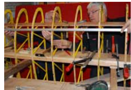
The wing ready for skinning the "D" box. Photo: Ove B. Hillersborg
