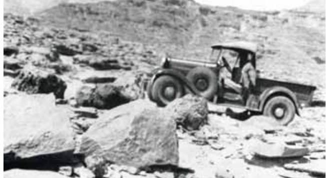
Ford trucks proved invaluable in the desert with the often difficult terrain. Taken at the foot of the Gifl Kebir; note the specially fitted balloon tyres to give extra grip in the sand. (East-Clayton expedition.)
