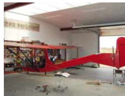
The newly restored 1949 "2G Primary" being rigged at the Lemvig Airfield in the North-Western part of Jutland in the spring of 2013. On this day new main pins were fitted and weighing performed. Photo by Ove B. Hillersborg.
