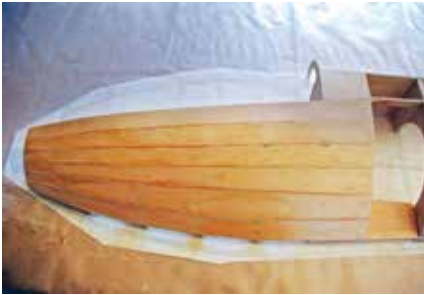
The fuselage nose was skinned in sections, using the 'crutch' method of assembly to produce a half shell
