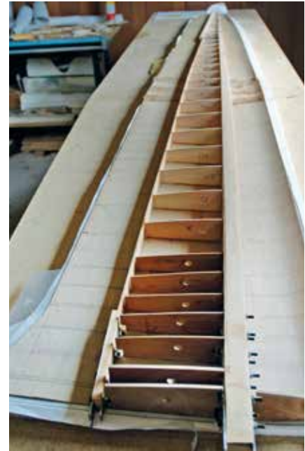
The wing skin of 0.4 mm plywood was laid into the female mould, the spars and ribs added.
