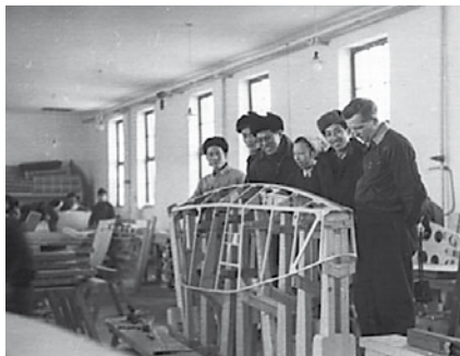
Fuselage assembly of a Chinese assembled Salamandra at the Shenyang sailplane works.
