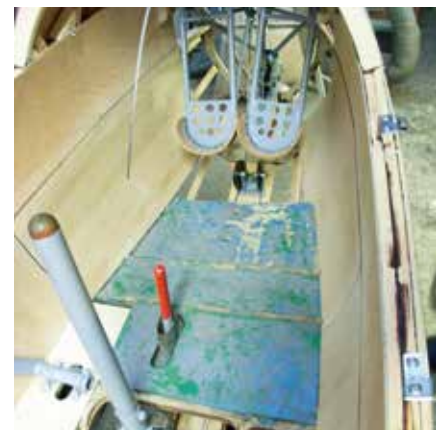
Cockpit details. Note the original floor pan.
