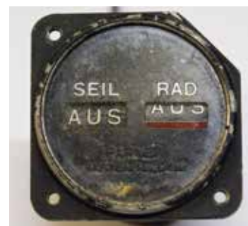
This device from Farmer, Grenchen, indicates the release status of the dolly and the towrope. Photo Thomas Fessler
