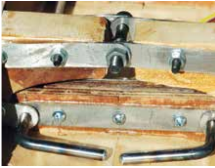
The re-designed main spar joiners.
