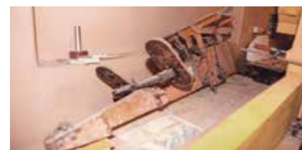
ABC glider during reconstruction, note the orange coloured fuselage structure of an original ABC which was used as a constructional template for the new fuselage in the foreground. Photo: Grzegorz Kazuro
