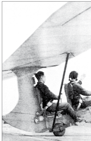
Jie Fang X5. Note the curvature of the rear kingpost, the position of the instructor's rudder pedals, and the attachment of the kingpost to the rear and front spars.
