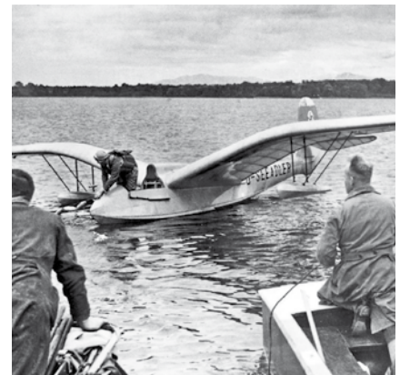
Floats were fastened to the tow line to prevent the rope from sinking.
