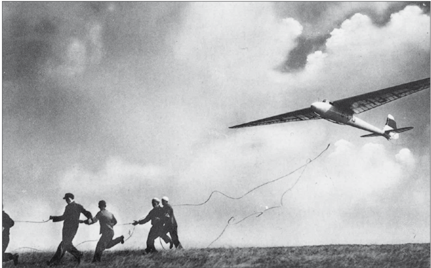
A Rhönadler being bungee launched at the Wasserkuppe. A well-known postcard, the photo was by R Büttner, via Martin Simons.
