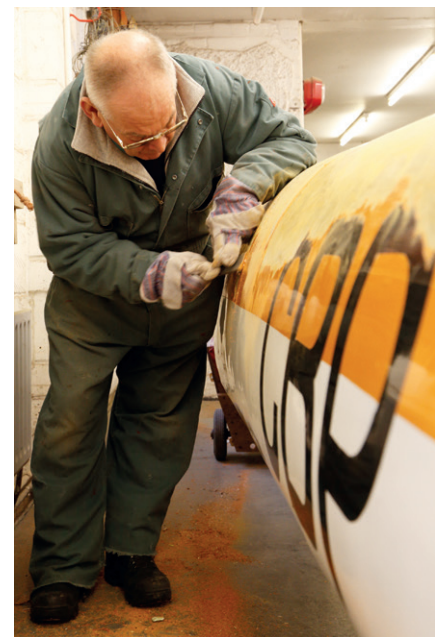
Ray Whittaker, VGC Membership Secretary, is hard at work removing the paint from the Foka Photo Paul Haliday
