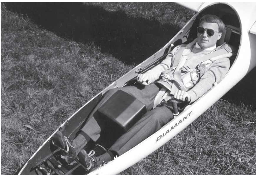
This photo shows the extreme reclined position of the pilot. Photo: Archiv Thomas Bircher
