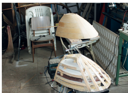
The Kite nose-cap takes shape, with the temporary jig in the foreground. Photo: David Underwood
