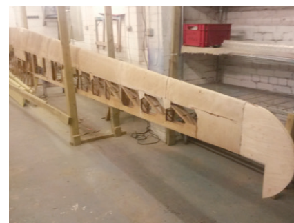
The newly restored port wing. Photo Mike Borrowdale
