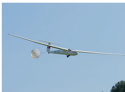
Brake parachute landing of the HBV Diamant HB-762 on the airfield Bad Ragaz on 4th September 2005. Photo: Martin Zahner
