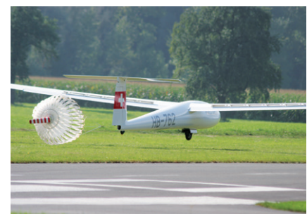
This photo shows the long brakes and the all-moving tailplane of the HBV Diamant. Photo: Martin Zahner
