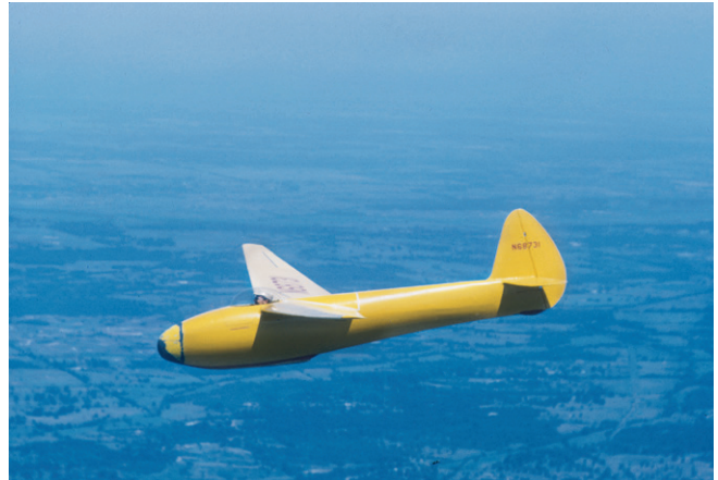
The modified Tiny Mite with increased wingspan, turtle deck removed and extensive smoothing and sealing
