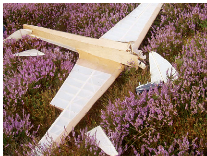
Oops!!! Never skimp on elevator control links.
