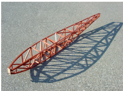
Fuselage basic structure. Photo Michael Kelly
