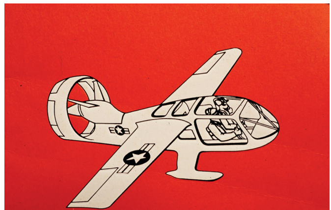
The Marvel. The first GRP Turbine-powered aircraft flown in the U. S.
