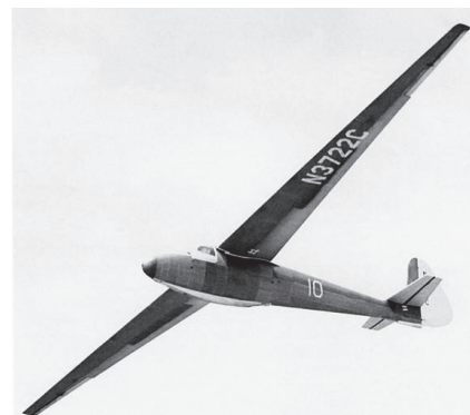
RJ-5 at Elmira for the 1951 Nationals (note the lack of a fillet between the wing and fuselage, much effort went into developing one but none provided a performance increase.)
