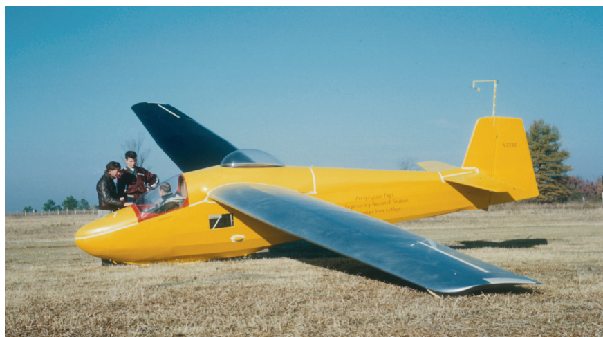
TG-3 modified to provide access for the Flight Test Engineer to the lower surface of the wing
