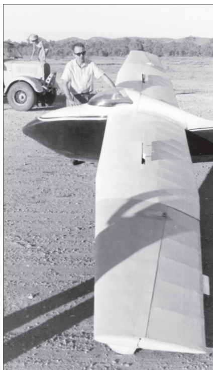
Now modified, the Swallow was renamed Swift. Pictured here at Mt Isa, note the enclosed canopy and airbrakes. Photo: Neil Hart via Bernard Duckworth
