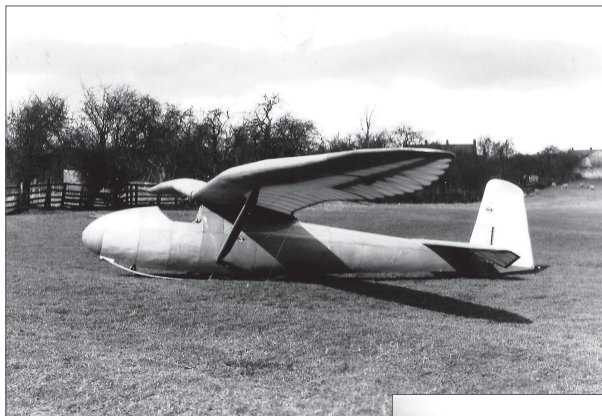
Early Kite, possibly the 2 nd or 3 rd produced (not the prototype as the rudder has a curved top). Photo: David Underwood
