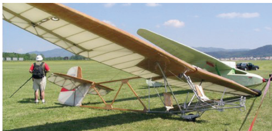
Roda dual-control glider with mixed structure, Yugoslavia, 1946. Span: 12,75m; best L/D: 15.
