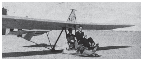
The two-seater Zögling which was a modified Bonomi Allievo B, Egypt, 1939 Span: 11,4m; best L/D with two persons: 12.
