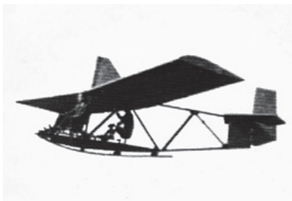
The modified AVIA XIA with an instructor seat built in behind the pupil and with dual-control. France, 1930-1933.
