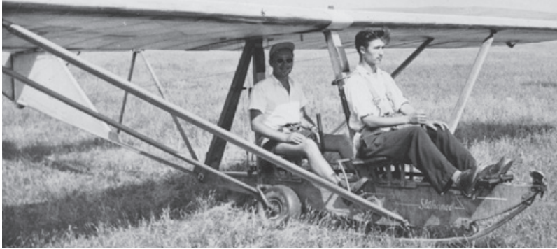
The RG-3 Stahanov. Rumania, 1953. Span: 12,6m; best L/D: 16
