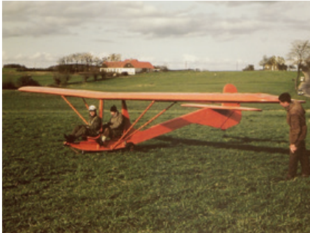
2G dual-control primary glider, Denmark, 1946. Span: 12,5m; best L/D: 13
