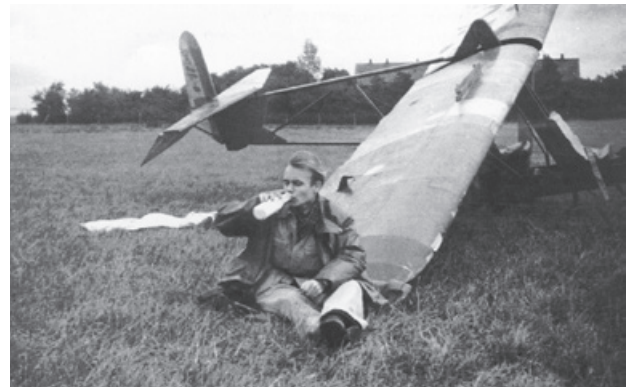
Vuggen two-seater. Span: 10,94m; best L/D: 12 (Original G-2 data)
