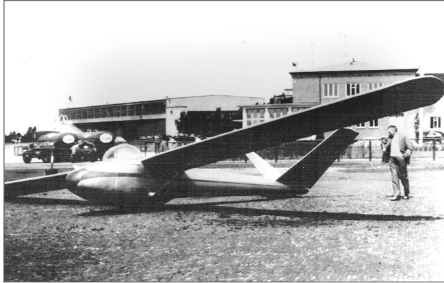
Photo of the 'Bremen Lane' taken at Bremen airport. The glider could be flown with an open or closed canopy. The closed one looked like a semi ball.
