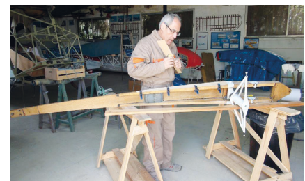
Working on the skid of the Vilanova i la Geltrú, Bergfalke, EC-FHL
