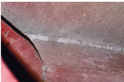
A sound casein joint in the GHC Viking 1. Note the glue-line in this photo still retains much of its original colour.
