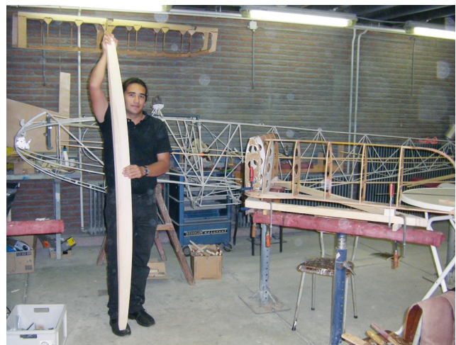
Justin Steegh shows off the newly constructed skid for the Ka3 fuselage in the background.
