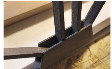
Well-preserved casein glue joints on a pre-war Slingsby Dagling wing rib. Photo: David Underwood
