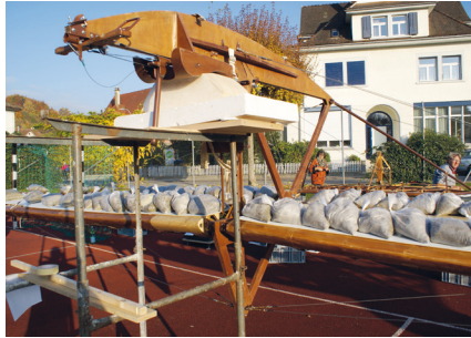
A nervous moment; load testing the Zögling's wing.
