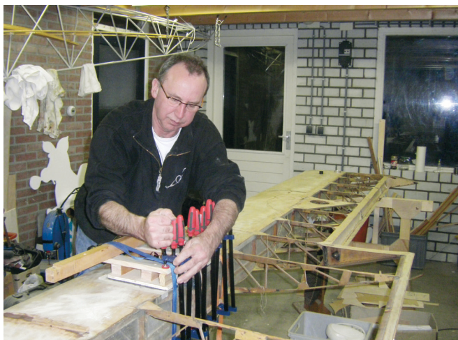
Johan hard at work play? Here he is working on repairs to Ka3, D-2397's port wing leading edge D-box.
