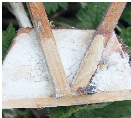
Prototype Kite 1. Nose rib with major breakdown of casein glued joint. Note the remains of the white fungus residue
