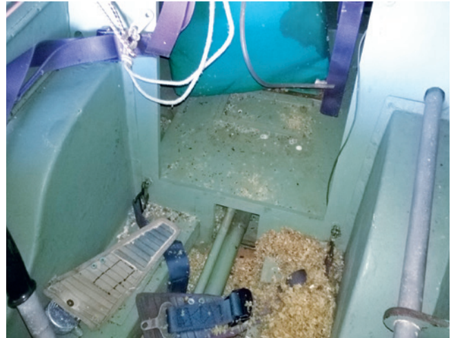
Rodent infested gliders will need thorough cleaning and deep inspections.
