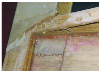
Freshly exposed Aerolite joints on a Capstan glider manufactured in 1964. Notice the similar appearance to Kaurit, however differs by showing up as a more solid colour/texture.
