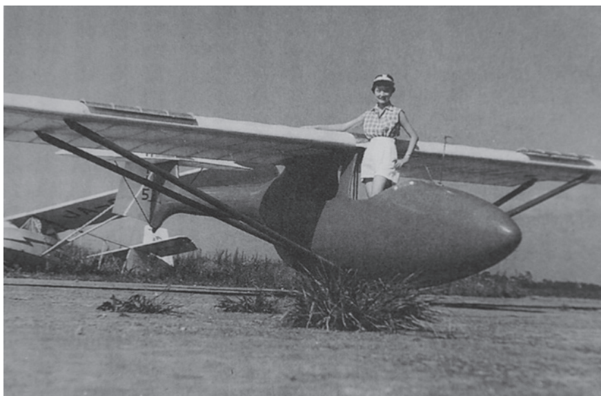
The University of Tokyo's (Todai) LBS-2, JA0115-1. Note the unique spoilers located in the leading edge of each wing, just inboard of the strut pickup points and proved largely ineffective.
