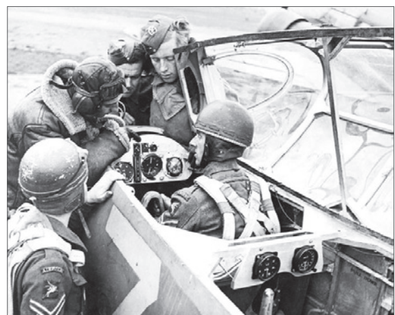
Mk III Training Hotspur. Note the addition of the instruments in rear cockpit. Photo via Dave O'Mally
