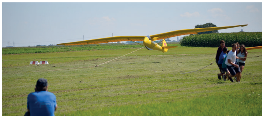
Bungee launch of the Spalinger S-19, HB-225, at Gundelfingen. As a slow-flying 1937 glider, it known as a perfect glider for bungee launching. Photo: Karin Lehmann
