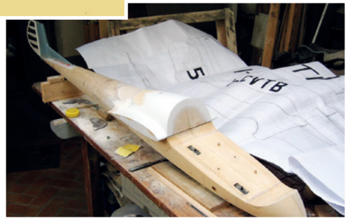
The wooden master mould for the fiberglass fuselage.
