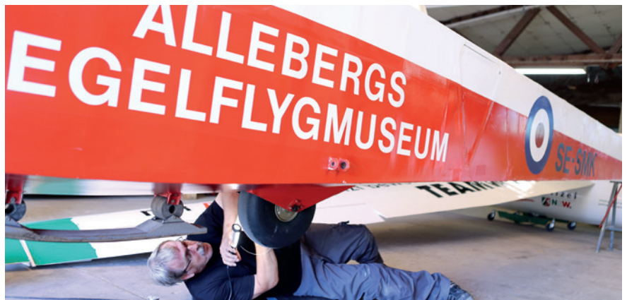
Petter Lindberg secures the wheel of the Slingsby T21. Photo: Thorsten Fridlitzius
