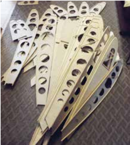
Major components of the wing have already been manufactured and only require assembly
