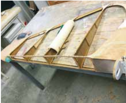
The Ka2 rudder after stripping back revealed a horror story of extensive Kaurit glue failure. The glider appeared to be in 1 st class condition but deeper investigation after substituting minor trailer damage revealed that even the most well-kept gliders were not immune from glue failure.
