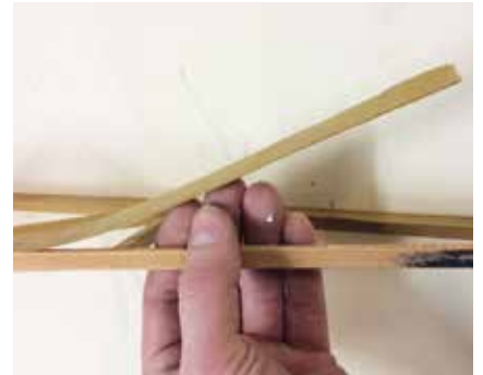
More classic cases of Kaurit glue failure, this time in a K8 wing. Again a well-kept example with no history of damage. As you can see from the photos above, classic glue failure with the wood simply being able to be peeled away. To say we were surprised at what we found during the inspection would be an understatement.
