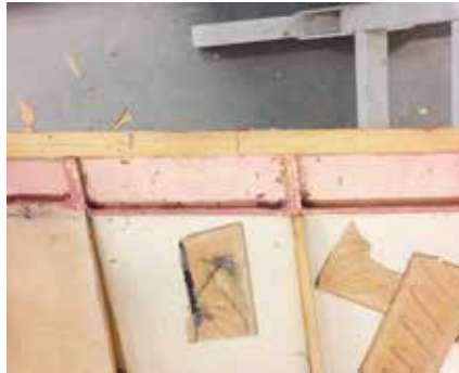
More classic cases of Kaurit glue failure, this time in a K8 wing. Again a well-kept example with no history of damage. As you can see from the photos above, classic glue failure with the wood simply being able to be peeled away. To say we were surprised at what we found during the inspection would be an understatement.
