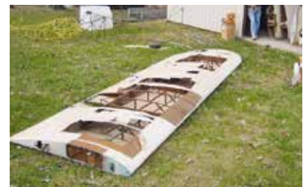
Old tattered fabric holding glue-failed ribs together for the trip home
