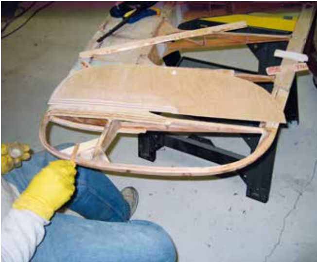
Applying Aeropoxy for Ka-2b wingtip repair.
