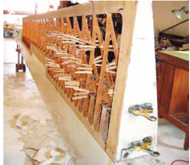
Using T-88 to glue half-round gussets on a Ka-6 wing. Note the generous use of clothespins as 'clamps'.
