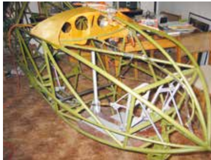
The use of steel tube and steel channel for fairing strips rather than wood guaranteed a rugged fuselage. Substantial rudder pedals were deemed necessary to push the huge rudder around..... in an age when pilots were expected to use their feet!
