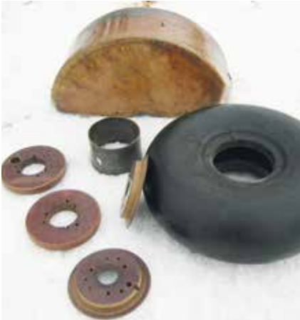
The original wheel built of Micarta (phenolic) in many pieces. The center spacer is a flat piece of steel formed to round. The original plywood wheel fender was reinforced all over with an extremely fine cloth, possibly silk, and a clear resin material. As much of this was retained as possible
