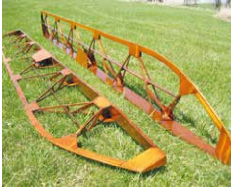
The ailerons are huge by any standards; 11 ft. long and 15" wide.
