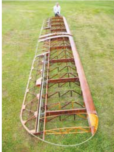
Very little new wood was required in the rebuilding of the wings, but all of it was re-glued. Note the older-style 2 spar wings (here fully restored) typical of so many American aircraft of the day, with D-box style wings in Europe having been standard for many years. As can be seen from the photos, the aesthetic beauty of the mahogany colour that the wings had naturally taken on over the years.
