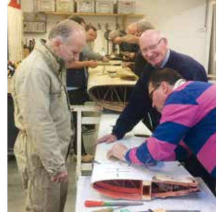
Hans Bekker persuades his students to make their plywood repair to a scrapped Ka6 wing upto airworthy specs.
