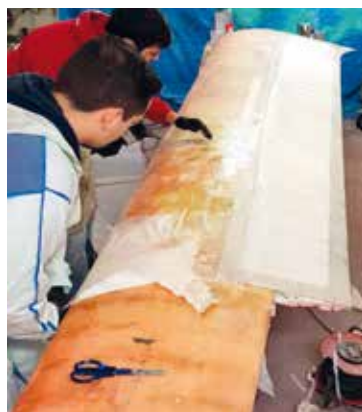
Glass cloth is being applied to the wing surfaces to reinforce them for alpine flying
