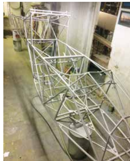
The Ka-4 fuselage stripped, sanded and newly painted
