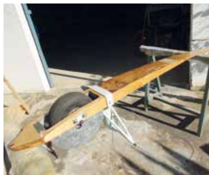
Wheel-box and skid of the Bergfalke, EC-HFL at the Vilanova y la Geltrú workshops.
