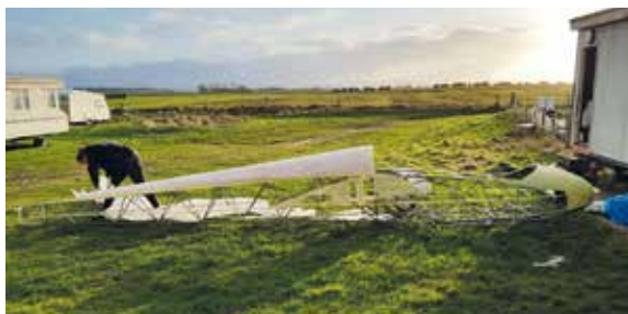
The bare bones of the K-13 as it is readied for soda-blasting
