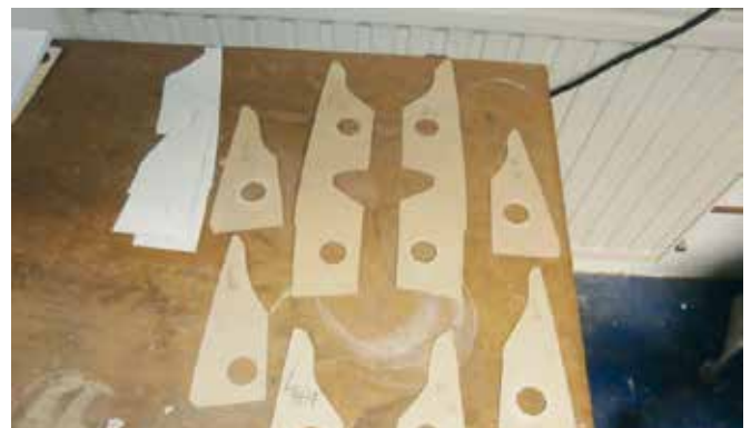
I was then able to cut new plywood gussets for each corresponding rib.
