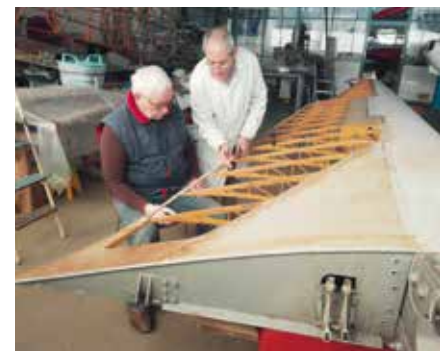
Hans Vom Hertel (left) and José work on repairs to the Ka-7 wings at the CCA workshops. Photo:
