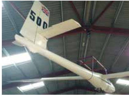
With a reputed glide ratio of 37:1, the only remaining KH-1 Scorpion's future is secured at the GHC. Photo: Paul Haliday
