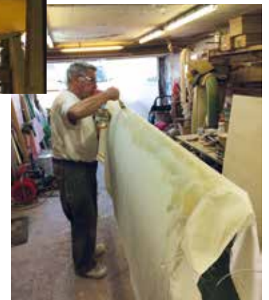
Peter Wehrli is covering the left wing of the Spalinger in cotton.
