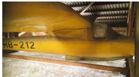
Peter Wehrli is covering the left wing of the Spalinger in cotton.
