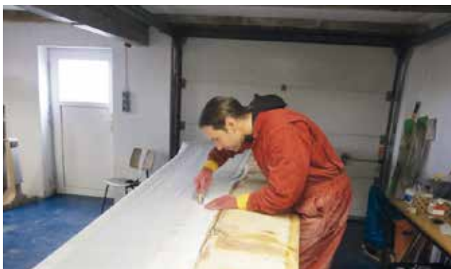
Cutting the edges of the fabric to shape using a roller knife.
