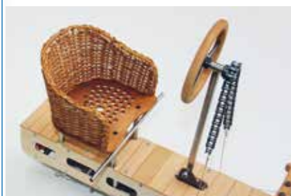
Some of the fittings now in place, all braced with 1mm control cable.
