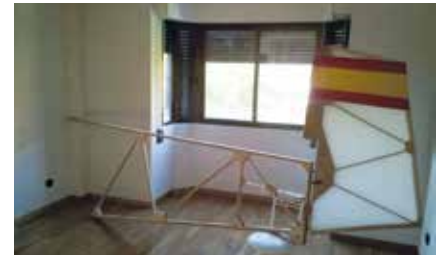
The SG-38 project of Carlos Bravo and Encarnita Novillo. The rear fuselage and rudder is largely complete.
