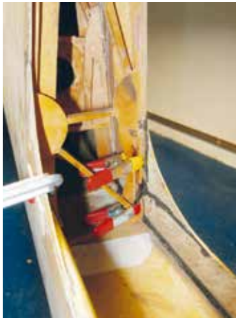
Few areas required any re-gluing.
