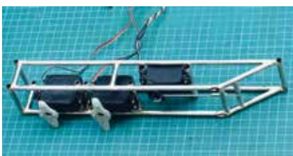
Some of the fittings now in place, all braced with 1mm control cable.
