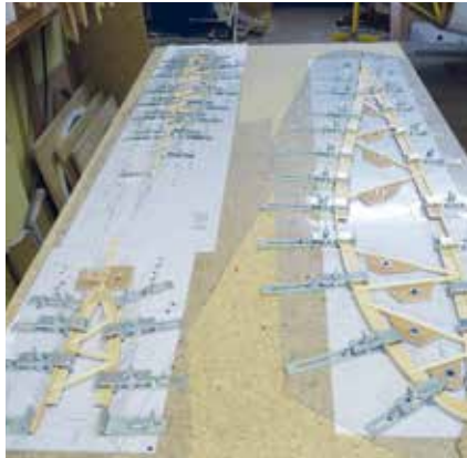
Even the wing-rib jigs are a work of art
