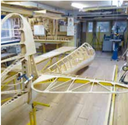
The rudder and elevator are trail-fitted for alignment
