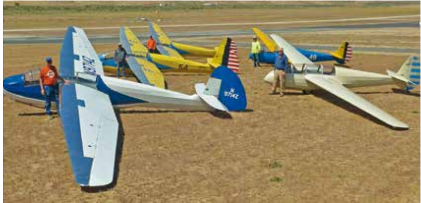
Vintage WW II two-seaters at Tehachapi Western Vintage and Classic Regatta. Front row SGS 2-8 and two Schweizer TG-2's. Rear row two Laister-Kauffman TG-4 / LK-10A's. Photo: Cam Martin.
