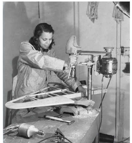
Earsly Taylor working on the tail-plane of the M-2 in their rented Detroit premises.
