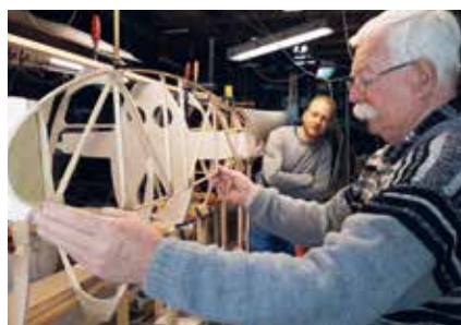
Aligning the fuselage formers with the spars of the wing
