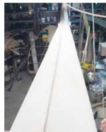
The plywood fitted to the top section of the aft fuselage
