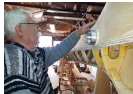
There is hardly a straight line on it! Skinning the aft section of the fuselage
