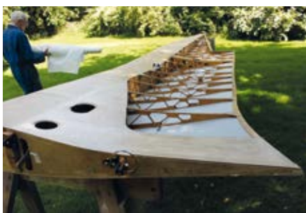
With the control cable in place, fabric goes on.
