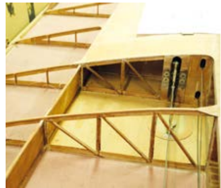
Wing construction details. Note the original DFS method of rib construction with the plywood gussets in the centre of the rib, making rib construction more complex.
