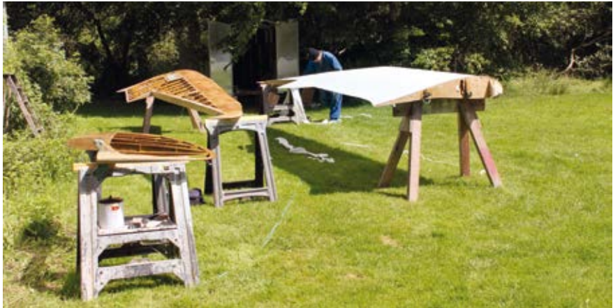
All coming to together nicely with fabric on the wings.
