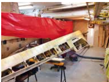
A deep inspection of the wings revealed very little in the way of any real work being needed as the covering process utilising Oratex begins.
