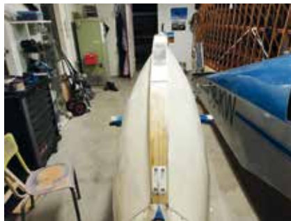
A new stainless steel skid for the Rhönbussard.
