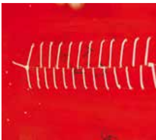
Basic fabric repairs are a must to keep hangar rash at bay.
