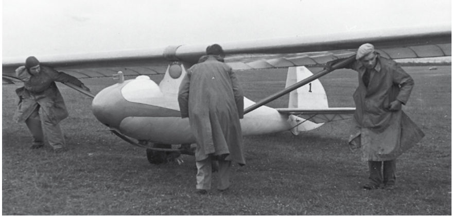
The Dart Cambridge at Dunstable with late VGC member, Mike Maufe at the left wing. Originally named the Zander and Weyl Cambridge, the Cambridge made its first flight a few months before Zander and Weyl Ltd. changed its name to Dart Aircraft Ltd. An updated version of the successful and influential Grunau Baby, the Cambridge retained the Baby wing, though with a slightly increased in span and utilising the popular Göttingen 535 of the Grunau. Owned by the Duke of Grafton (who was a Cambridge GC member), it was flown as a club aircraft and was entered into the 1939 National Soaring Contests, though without distinction. A little later on a Cambridge II was constructed which utilised slightly larger ailerons and was operated by the London Gliding Club who flew it into 6 th place in the 1937 National Competitions. The Cambridge 1 survived the war but was later wrecked in a collision with an Olympia at Camphill in June 1952, with the demise of the Cambridge II coming in 1967 by being burnt.
