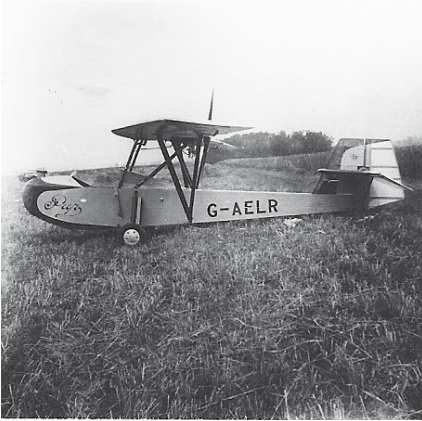
The 1936 Dunstable Dart, which became the Dart Pup during its construction process, proved to be a versatile design with an Avia flat-four pusher engine mounted on the wing trailing edge. The wings could be folded back for storage. In August 1938 it crashed and was destroyed on takeoff.
