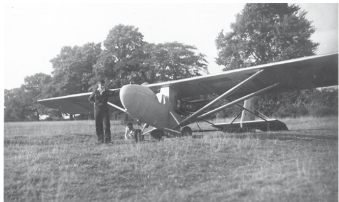
The Flittermouse was powered by a 25 hp Scott Squirrel engine with a pusher propeller. Although it proved a popular aircraft with its owners, there was only ever one aircraft built and registered G-AELZ. After a number of private owners it was scrapped at Blackbushe Airport in 1951.
