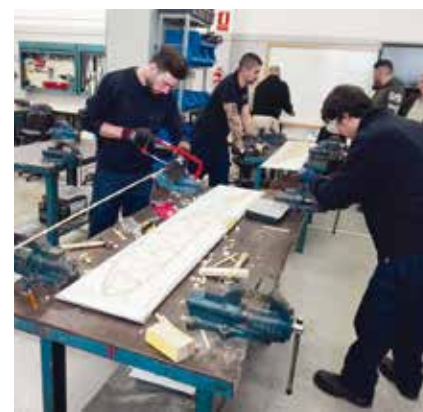
Old skills for new hands... apprentices at the Aviation School at Vilanova y la Geltrú building SG-38 ribs.
