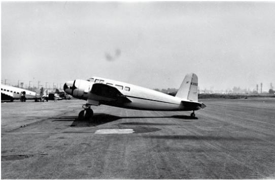
The Bennett BTC-1 Executive Transport, an 8-passenger corporate plane and first composite aircraft. Source: Internet
