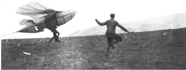
'Senator Zeise' glider with the pilot Theo Suchla. The member of the Halle Aviation Association died as a police lieutenant in the 1921 March fights. Zeise's glider consisted of bamboo, plywood and oiled silk as covering material. The tethered take-off took place on short ropes on the outer wings, and the pilot struggled to land safely on his feet after a short jump. The wonderfully crafted aircraft received a 700 mark prize from the Kyffhausen technical centre for the best and lightest construction of a closed fuselage with maximum strength and weather resistance, as well as 300 mark for the cleanest glider. Photo: German Glider Museum
