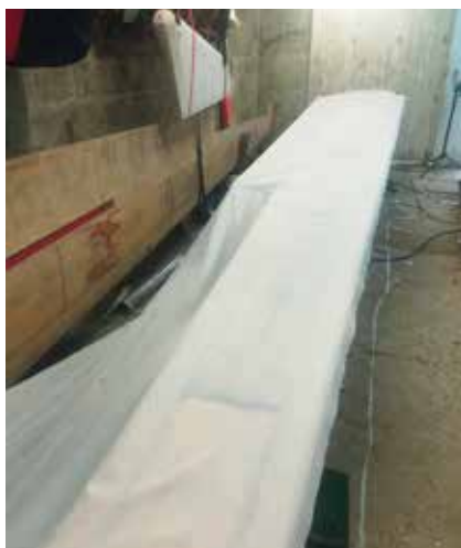
The Pik's wings are now covered. Photo: Benoît Auger
