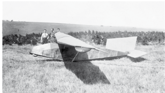
Photo Caption: The Vampyr was a revolutionary design with its pneumatic undercarriage and a single-spar, stressed skin plywood D-box wing which set the trend for decades to come. Photo: Martin Simons, Sailplanes 1920-1945, Equip Verlag, Bonn, Germany
