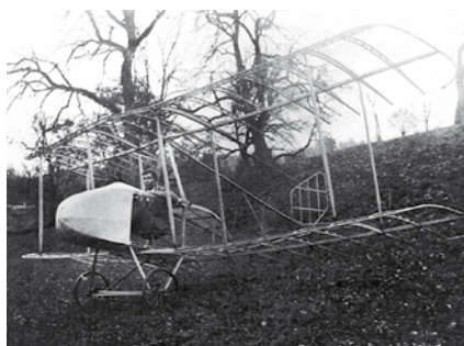
The Spalinger S-1 appears to be a biplane without an engine. Photo: IG Albatros archives
