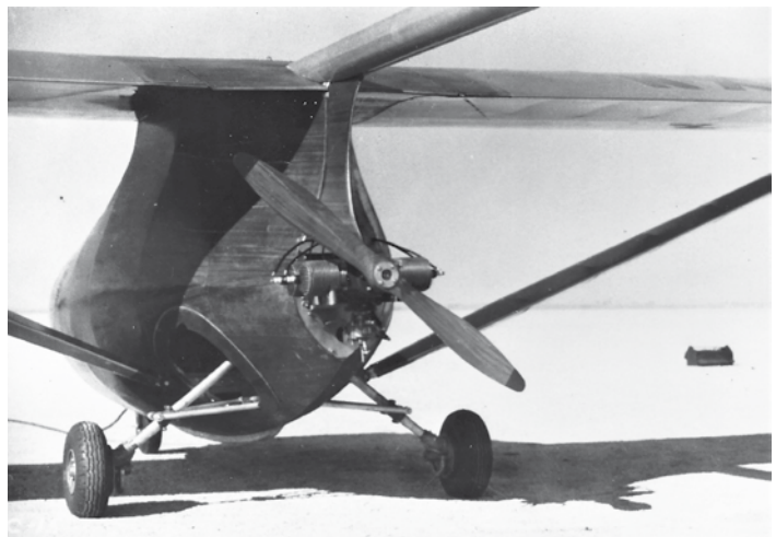
The BB-1 Bumblebee engine installation. This was typical for the Dragonfly too. Photo: Dick Benbough
