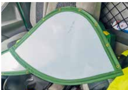
Preventing flies one's teeth, these new windscreens are a welcome addition to the dwindling availability of T21 spares.
