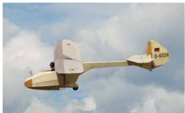
The Cumulus IIF is not fitted with airbrakes to assist the approach for landing. Photo: Frank Henze
