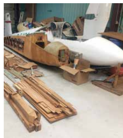
Neal Pfeiffer's newly-discovered, unfinished and unflown kit Slingsby Swallow. The kit is shown unloaded in Neal's shop. Behind is Neal's Ka-2B project. Photo: Neal Pfeiffer
