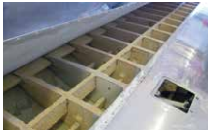
Details of the wing construction detailing the inner structure of the wing. Photo: Walter Linden
