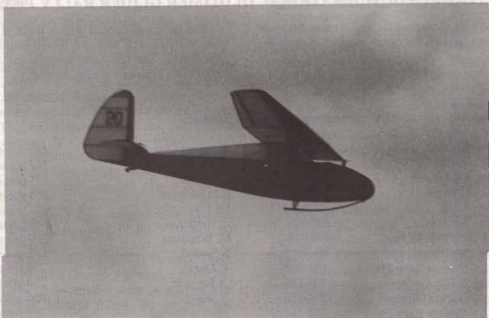
PEGASUS flies again. A 1/3rd full size model by Peter Saunders, who also took the photo. 11ft 4" span. Wing Loading 14 3/4 ozs/sq. ft. The original flew in 1935. Only one was built. Span 1.47 m. Empty weight:- 135 lbs (61.23 kgs). Max. L/D 1/20.5. Wing Profile Goe 535. BGA 232.
