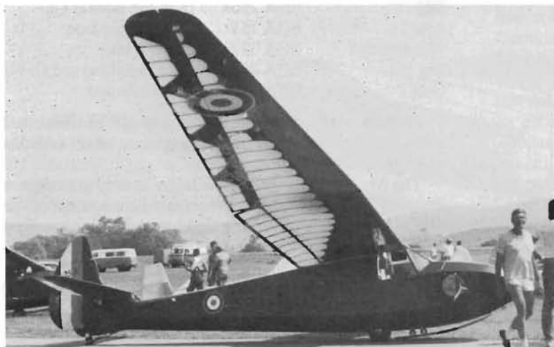
The magnificently rebuilt and recovered Castel C 25 S. So far as we know it is the first French glider to be restored with transparent fabric. Its restorer and owner, Jean Paul Robin, can be seen walking by its nose. VGC Restoration Prize 1989.
