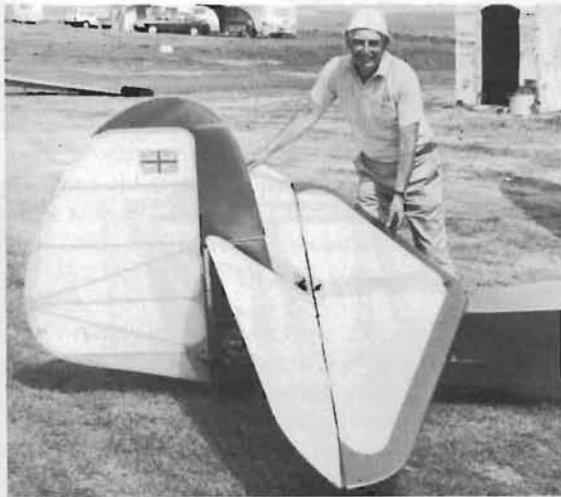
Murray Hayes tests elevator movement of his postwar Naval Dockyard built Grunau Baby 2b which has a Kite 1 type rudder and tailplane. This aircraft and its owner had distinguished Royal Naval careers.
