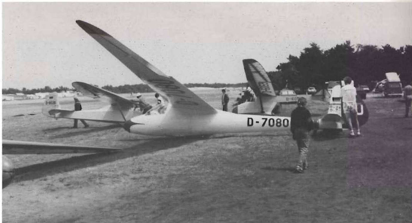
The Weihe which consistently gains first performance prize at our internationals, flown by Werner Tschorn. This was originally a French VMA 200 Milan (one of 30 built in 1950) which Werner rebuilt, using FW Weihe drawings. This year he flew two 300km triangles with it.
