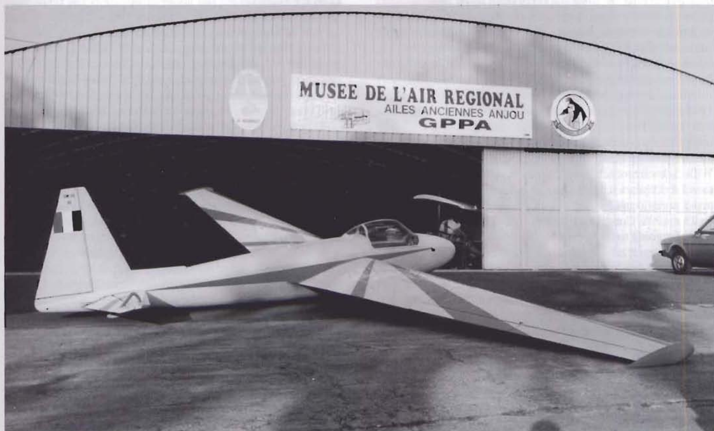
The 1949 NACA 230 wing profiled unique Fougas CM-8-13 which has just been restored by the GPPA at Angers for the Musée de l'Air et de l'Espace at Le Bourget. It is to be flown this year. It is fully aerobatic but has also a good cross-country performance.
