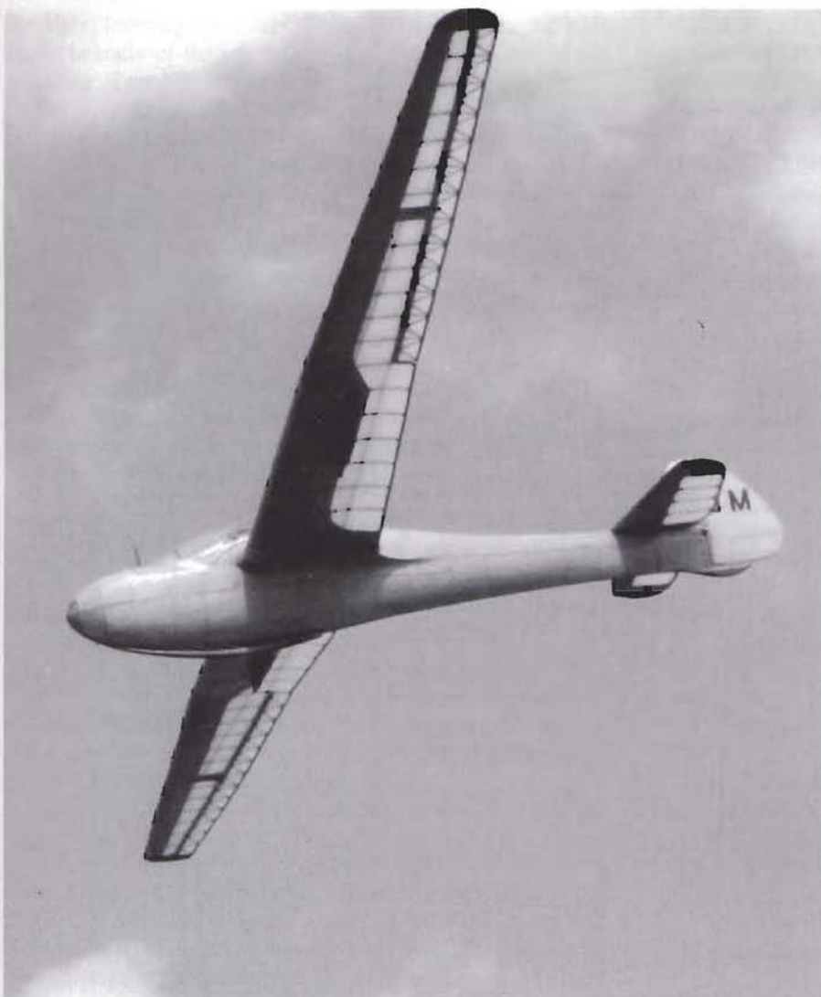
The Huetter 28-3, built by Earle Duffin, flying over the Wasserkuppe in 1995. Earle modified the design of the 28-2 (with BGA approval) to be more like the 28-3 for his greater comfort.
