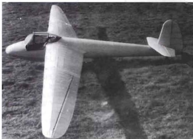
A swing-wing glider in 1944 with twin, retractable wheels! The Hirth 21, with the wings swept forward.
