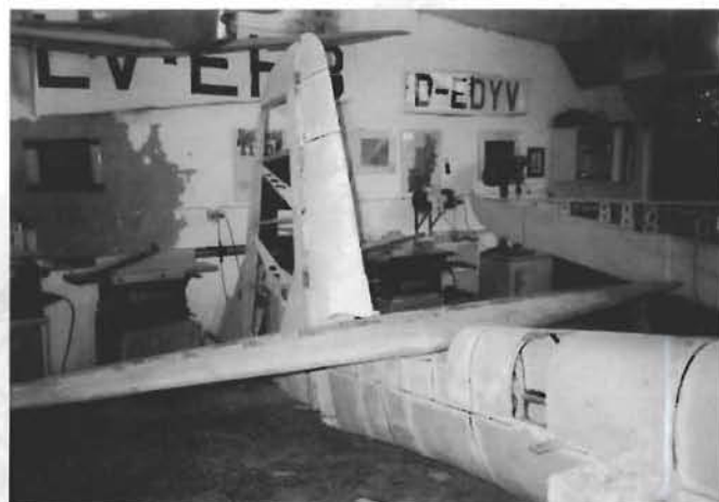
At Achmer/Osnabrück this Kranich 2 is being built from the remains of BGA 1092 fuselage and BGA 1258 wings and tailplane. Photo Manfred Hermeling
