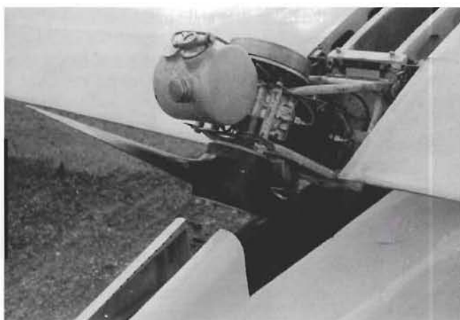
The innovative engine installation on the Beynes Scud 3 of 1935 when it was known as the Carden Baynes Auxiliary.
