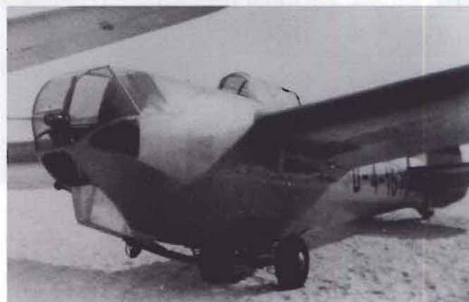
The Kranich 2 modified to have a prone pilot in the front only at Schönhagen.
