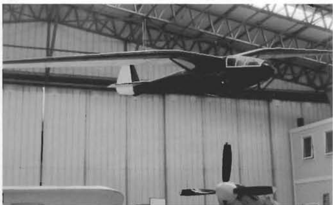
A Gull I (BGA 379, G-ALPA) made from several aircraft including the elevator and struts of Geoffrey Stephenson's cross channel Gull, at the East Fortune Museum.
