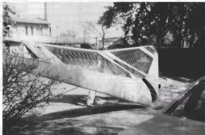
The framework of a Horten Piernifero 2, believed to be in Argentina. From C.Wills
